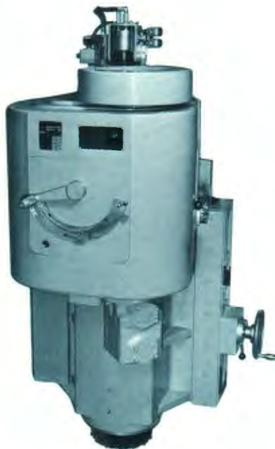
POWER PACK Overall Dimensions without Electric Motor 40" x 92" x 50" High 1016 x 2337 x 1270 mm
