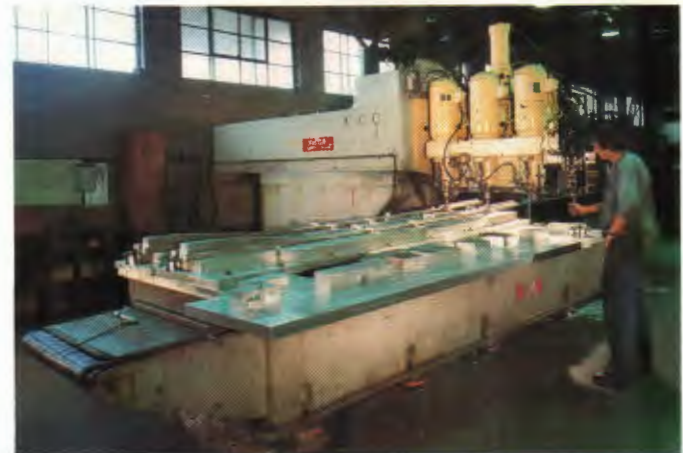
4 Spindle Havlik Profiler work area 40" x 72" per spindle.
