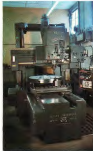
#6 Zip Jig Boring Machine with optics and work area 36" x 36".
