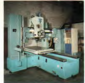
VR5N - N/C Drill, Bore & Tapping Machine - work area 36" x 48".
