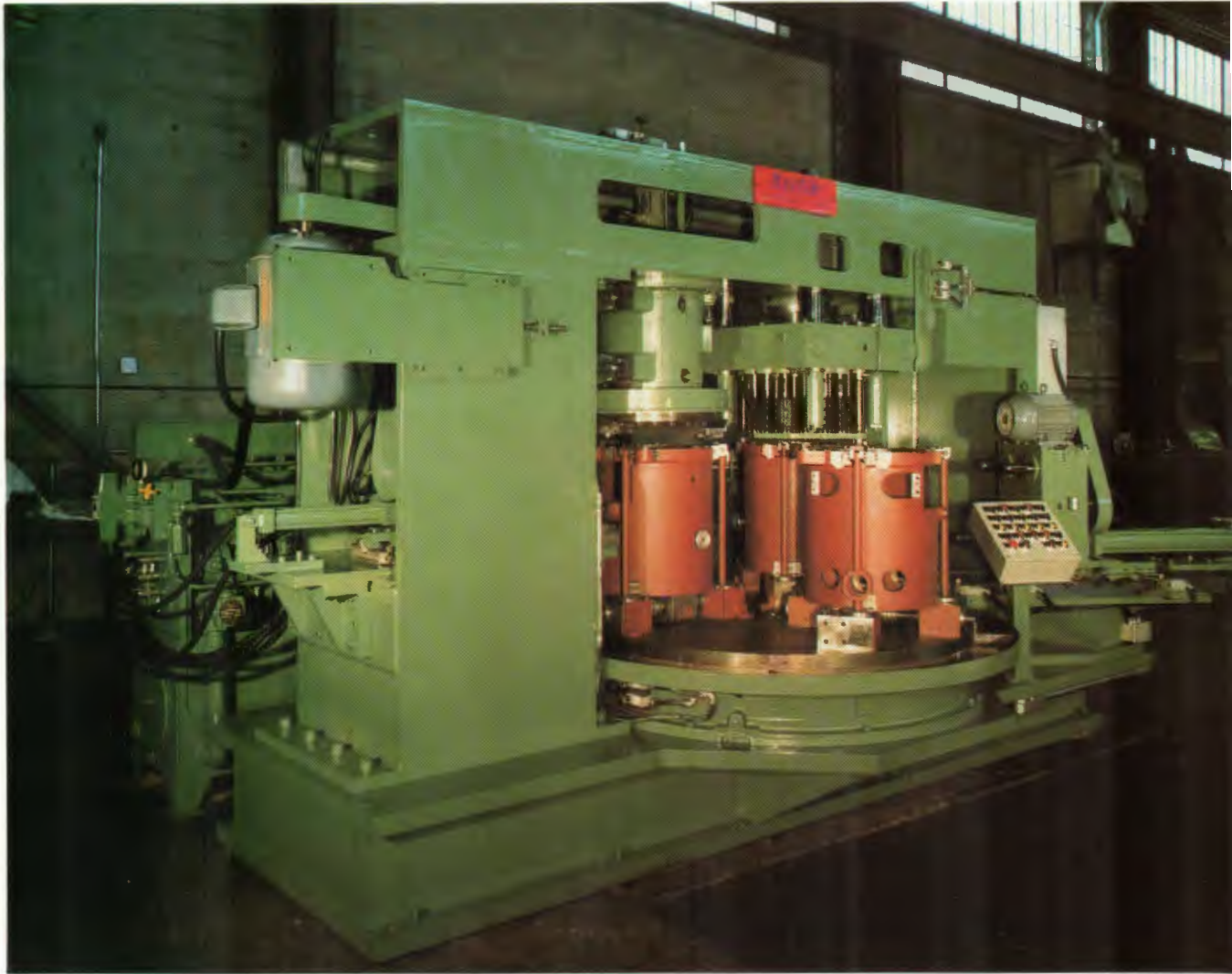
A special purpose machine built by our company for the drilling, facing and tapping of housings for air brake manufacture.
