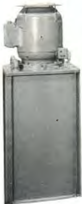
POWER PACK Overall Dimensions without Electric Motor 40" x 92" x 50" High 1016 x 2337 x 1270 mm
