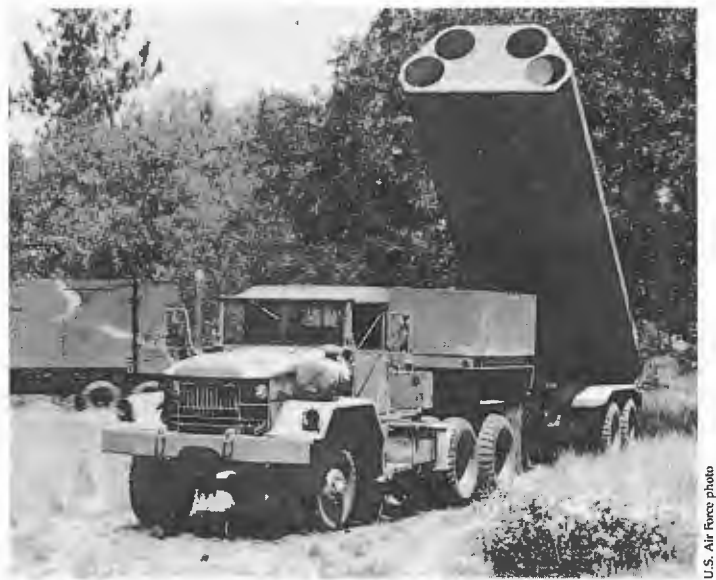
In foreground is a four-missile transporter-erector-launcher of the type used for U.S. ground-launched cruise missiles (GLCMs) in Western Europe. Truck in background houses launch control center.
