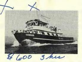
Launched in June 1979, the 88 ft. **CONDOR** is one of the country's largest and most comfortable sportfishing boats. Powered by twin 500 hp Diesels this boat has the speed and size to take you in comfort to the finest fishing grounds on the coast. The boat is equipped with all the latest radio, navigation and fish finding apparatus.
