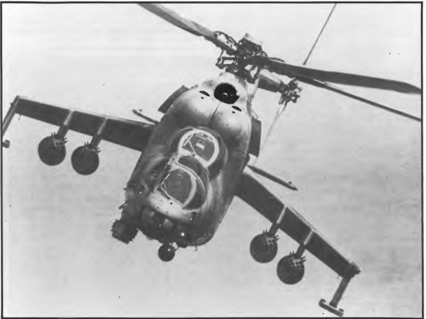
The Mi-24/HIND D (above and below) is one of the world's most advanced attack helicopters. It has a nose-mounted Gatling-type machinegun and can carry up to 4 pods containing nearly 130 57-millimeter rockets as well as antitank missiles or bombs. This is the same helicopter being used by the Soviet Union against Afghan rebels. The Sandinista air force now has five to eight of these flying "tanks."
