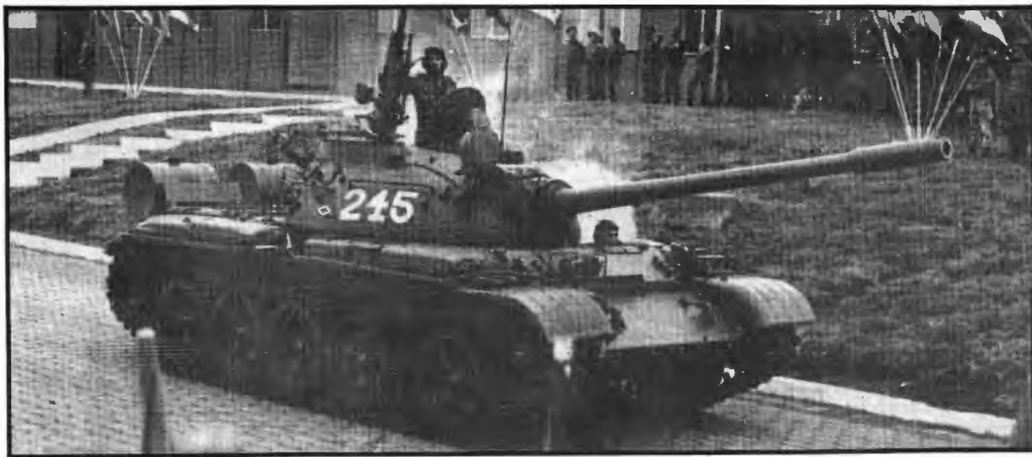
The Soviet-made T-55 tank weighs 36 metric tons and has a 100-millimeter gun. Formerly the Soviet Union's main battle tank, it is far superior to any other tank in Central America. The Sandinistas have more than 110 T-55s. In comparison, Somoza had three operational World War II vintage U.S. tanks.
