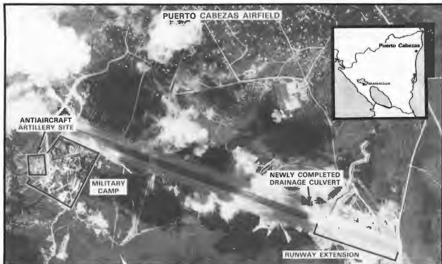
The Sandinistas are upgrading the airfield at Puerto Cabezas and lengthening the runway by more than 1,500 feet.
