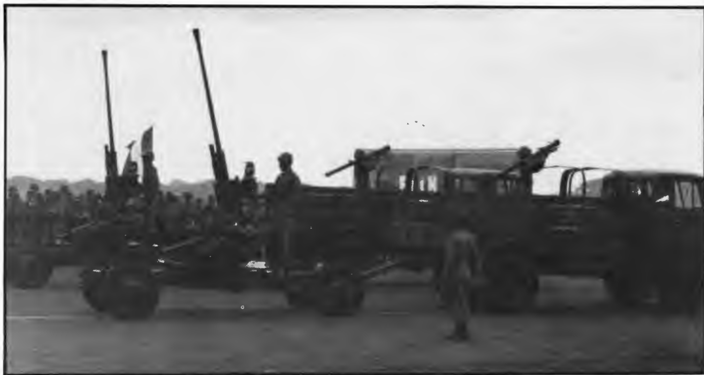
The M-1939, a 37-millimeter anti-aircraft gun, can fire at the rate of 160-180 rounds per minute. It has an effective range of more than 8,000 feet. There are nine M-1939 sites in the Managua area alone. Notice that in the bed of each truck, a soldier holds an SA-7 missile launcher.
