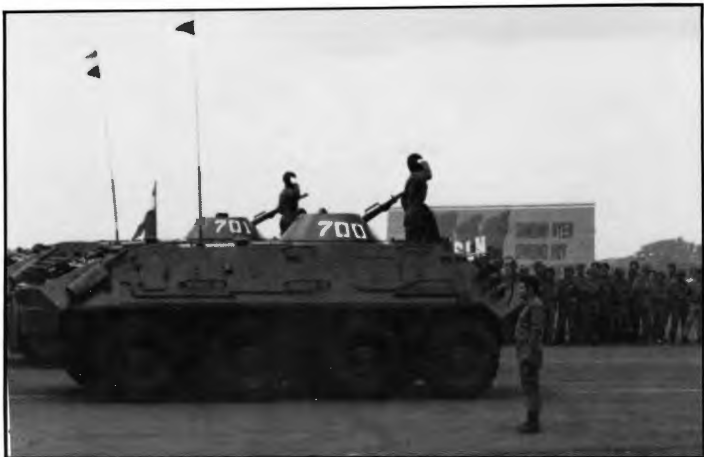
The BTR-60, an armored personnel carrier, can transport a squad of infantry. It is armed with a machinegun and is fully amphibious.
