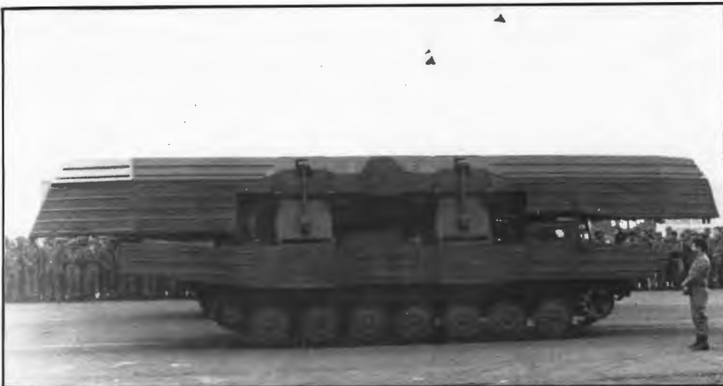
The Sandinistas have six GSP amphibious ferries which can carry heavy vehicles, including T-55 tanks, across rivers.
