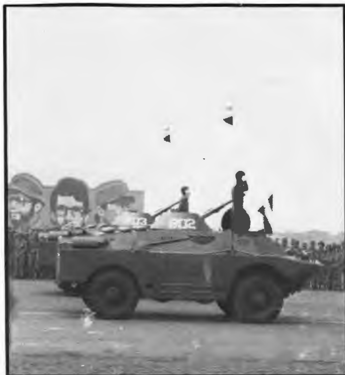
The BRDM-2 armored reconnaissance vehicle is fully amphibious and armed with a machinegun. The Sandinistas have dozens of these vehicles which, like the PT-76 light amphibious tanks and the BTR-60 armored personnel carriers, are well suited to the rough terrain in parts of Nicaragua.
