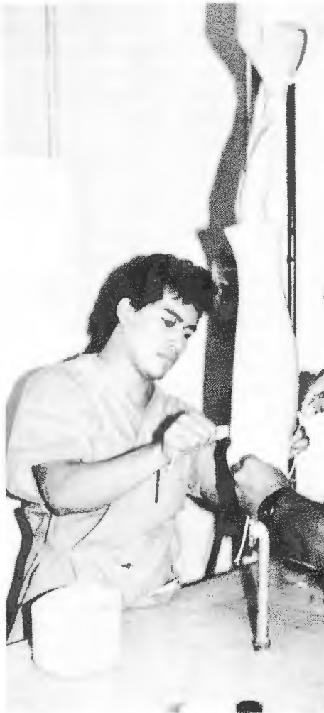
CERPROFA trainee laminates an artificial leg. The trainee, who was wounded by a guerrilla land mine, made his own prosthesis.
