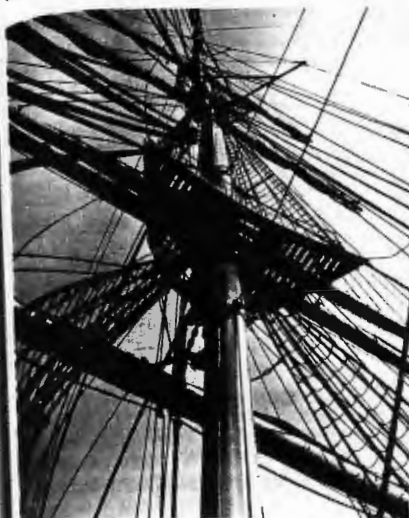
standing and running rigging showing mainmast, blocks, and junctions with shrouds and ratlines
