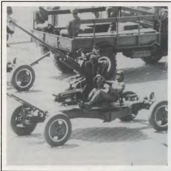
The M-1939, a 37-millimeter anti-aircraft gun, can fire at the rate of 160 to 180 rounds per minute. There are nine M-1939 sites in the Managua area alone.
