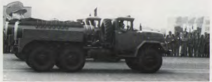
These ZIL-131 trucks, when equipped with decontamination tanks, can be used for chemical warfare.
