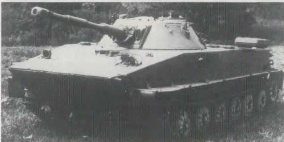
The PT-76 has a 76-millimeter gun and is fully amphibious. The Soviets provided the Sandinistas with about 30 of these light tanks in 1984.
