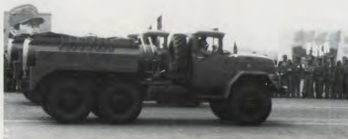
These ZIL-131 trucks, when equipped with decontamination tanks, can be used for chemical warfare.
