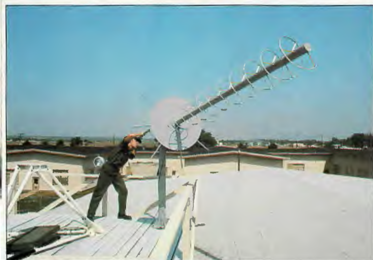
TOP: Hammer Ace consists of 11 suitcase-size units weighing a total of 375 pounds, providing mobility, security, and flexibility of operation.
