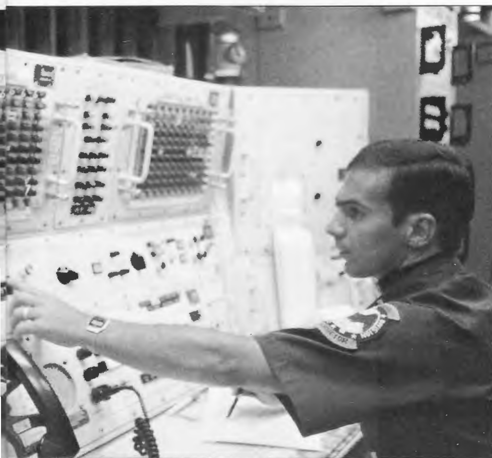
FAR LEFT: A Minuteman missile is launched from Vandenberg AFB, Calif. where combat crews are trained before assuming their duties in the field. LEFT: First Lt. Phil Anthony works at a console that has a series of alarms, lights, and computer printouts to warn him of any status change in the missiles or support equipment.
