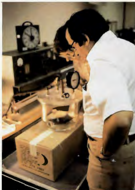
Left, Bill Hemstedt machines a parachute release to be used on a cargo parachute during an air-drop test. • Ted Ciavarini, foreground, and Jim Beyer watch for possible leaks in a Meal, Ready-to-Eat, package being tested in a device that creates a vacuum.
