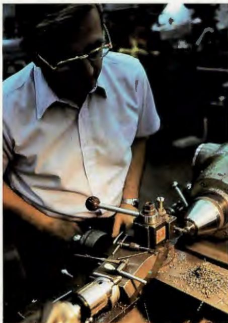
Left, Bill Hemstedt machines a parachute release to be used on a cargo parachute during an air-drop test. • Ted Ciavarini, foreground, and Jim Beyer watch for possible leaks in a Meal, Ready-to-Eat, package being tested in a device that creates a vacuum.
