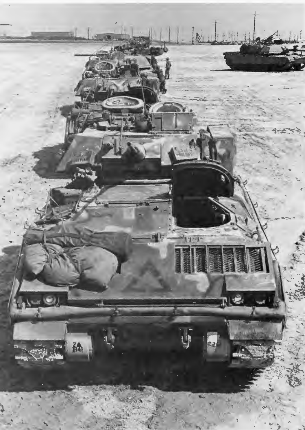
The M-2 offers equipment that includes a stabilized turret and an integrated day and night sight. Crews can shoot the turret weapons on the move and remain on target. At night, they can switch on the night sight and continue firing. They can also use the sight during the day to shoot through haze, dust or smoke screens.
