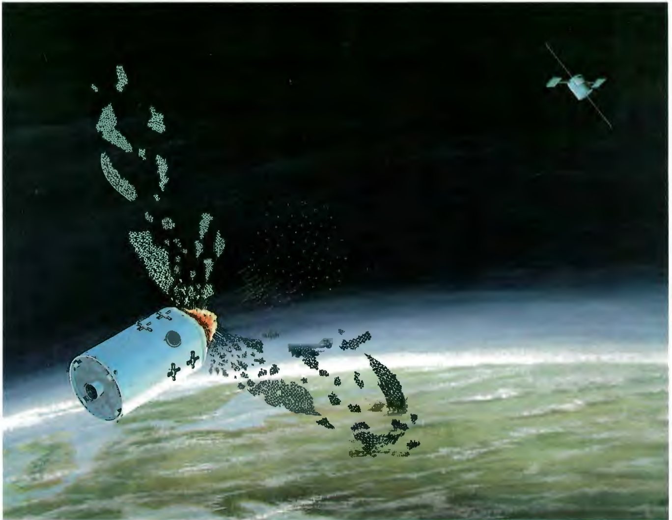
The Soviet orbital antisatellite (ASAT) weapon is operational and designed to destroy space targets with a multi-pellet blast.
