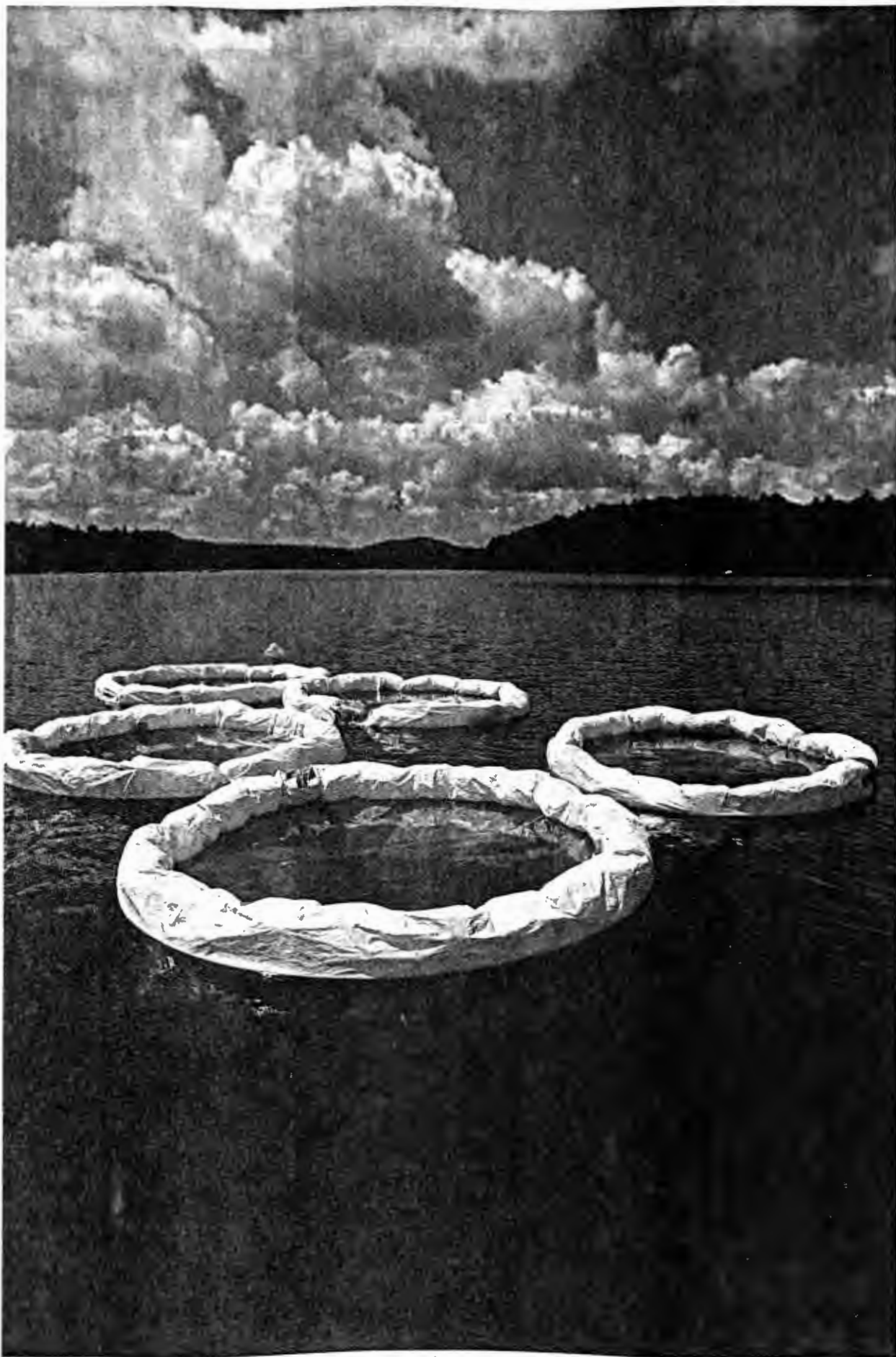
Big Moose Lake, one of the 200-odd Adirondack lakes that have been heavily acidified, has also been heavily researched. Syracuse University scientists use the "cylindrical columns" at left to isolate portions of the lake water so that it can be chemically tested without leaving its natural environment.
