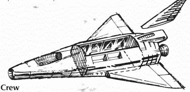
Both booster and orbiter have crew compartments. The booster's accommodates two pilots who will return the craft for landing. The orbiter also has a crew of two to navigate returns, but it will also be able to carry up to 12 passengers. The cabins in both will have a shirtsleeve environment, wherein spacesuits will not be necessary, which will be served by an atmosphere of oxygen and nitrogen.
