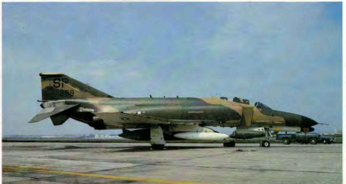
F-4G "Advanced Wild Weasel" A modified F-4E with sophisticated electronic warfare equipment
