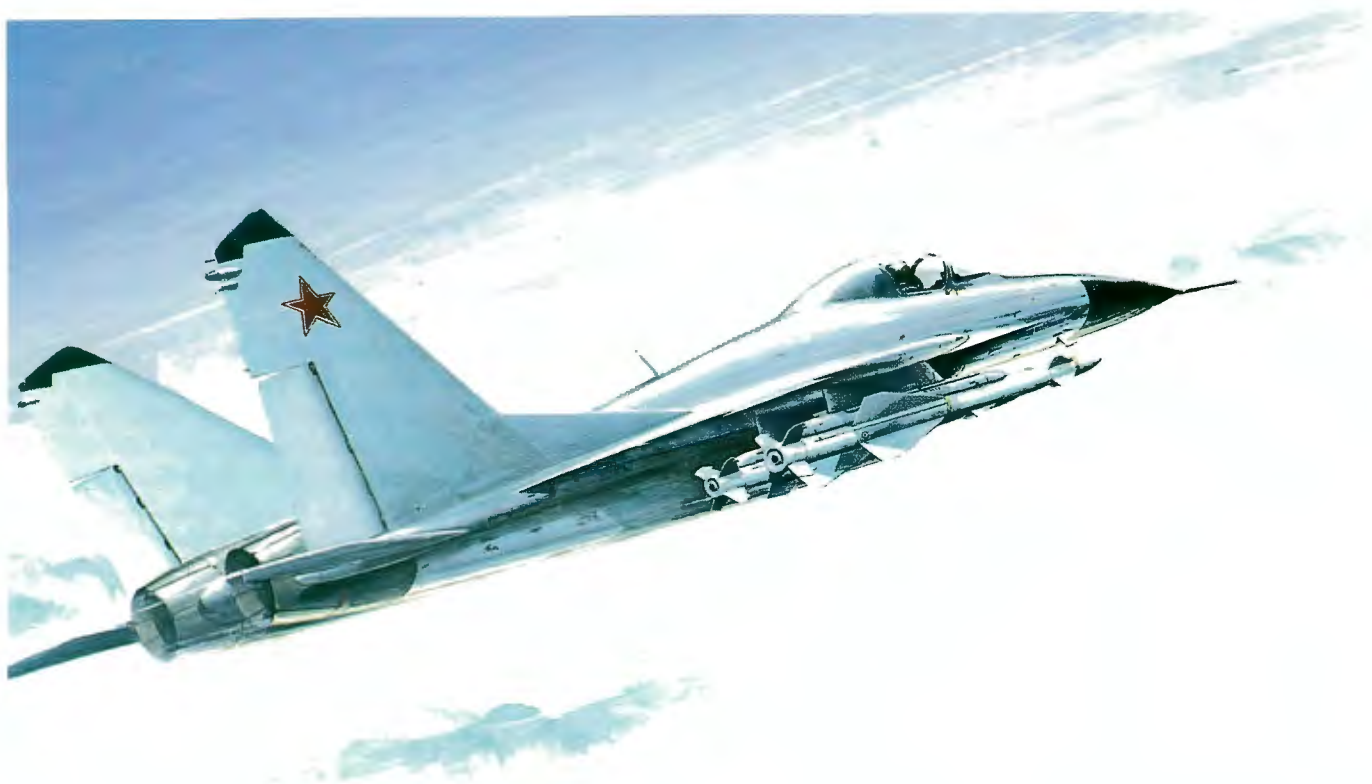
The MiG-29/FULCRUM all-weather, air superiority fighter-interceptor reflects the USSR's continuing drive to produce new generations of tactical and strategic aircraft. The FULCRUM is fitted with AA-10 missiles and the USSR's most modern look-down/shoot-down radar.
